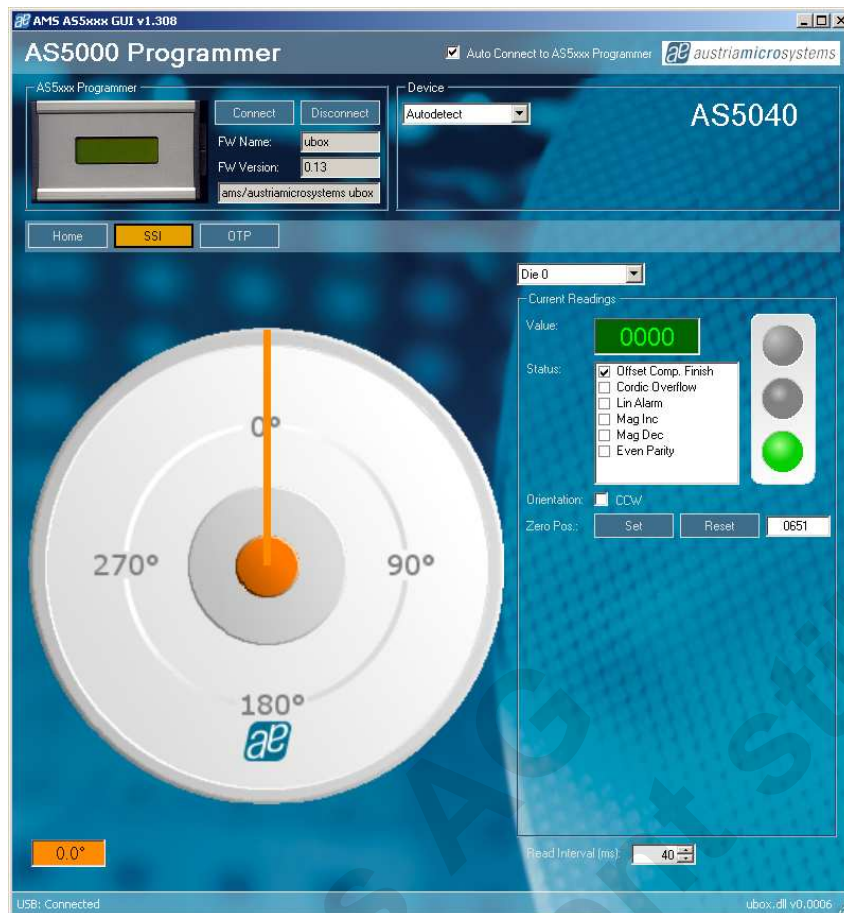
Figure 7: AS5040 SSI tab after Zero Position programming
